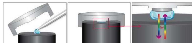
Fig. 2. Sample Compression Technology™ used in the NanoPhotometer™ Pearl.
